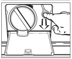
Pull the emergency release downwards. The door will open.
